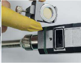
2. Take out the protective lens holder
