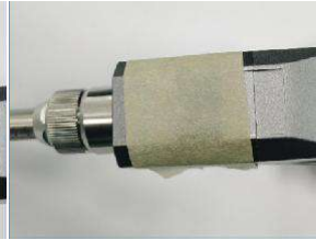
3. Masking paper package to protect the lens seat cavity
