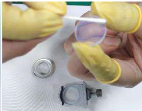
5. Take out the protective mirror holder and wipe the other side of the protective mirror
