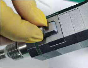
1. Loosen the locking screw of the protective lens holder shell
